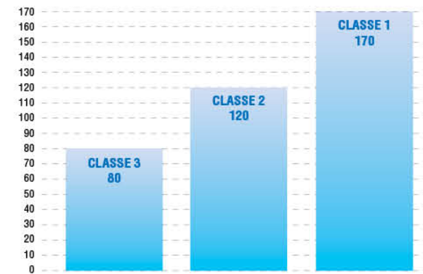
Classes defined by Regulation EN 676 for NOx emissions with natural gas
